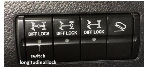
The centre-differential lock can only be switched on under the following conditions:
