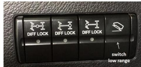
The Gear reduction supports when driving on difficult ground. There are 2 shift ranges available: road drive and gear reduction for driving on difficult ground.
