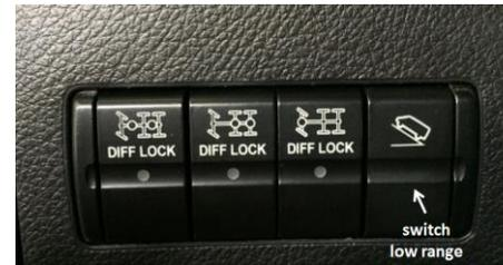
The Gear reduction supports when driving on difficult ground. There are 2 shift ranges available: road drive and gear reduction for driving on difficult ground.
