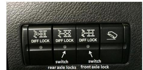
The axle-differential locks can only be switched on under the following conditions:
