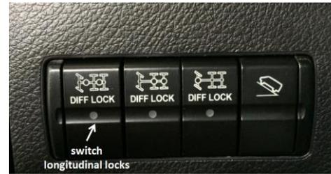
The longitudinal lock can only be switched on under the following conditions:
